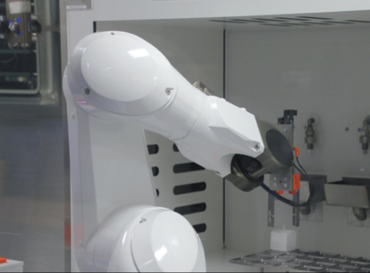
Six identical Stäubli Stericlean robots handle the implants. Shown here is the chemical treatment station.
